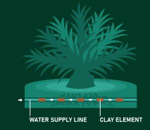
The concept, production and installation of the technology are simple and thus adaptable to rural environments. This technology is piloted in Gozo (Malta), Portugal and Morocco.
